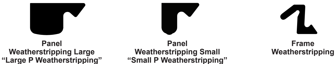
FIGURE B.2: PANEL WEATHERSTRIPPING PROFILES
